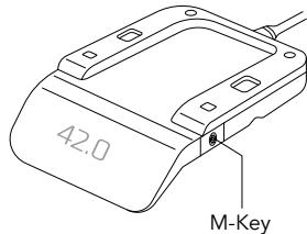
Press and hold the M-Key [ ] to access the [ ] menu. Then press the M-Key a second time to open the sub-menu [ 30 min ]. In the sub-menu, you can switch the timer on/off or select the time by pressing the handset up or down. Press the left [ ] key to go to the timer display. The timer counts the time during which the ofinto Rise is set below a height of 90 cm (sitting position). As soon as the set time has elapsed in a position below 90 cm, the handset will vibrate.
